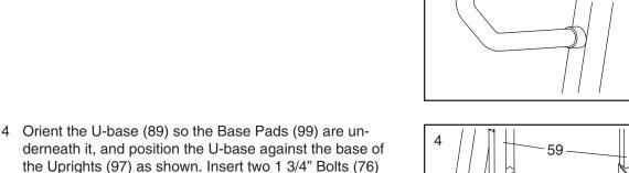
Next, insert two 3" Bolts (86) into the U-base (89) and the base of the Uprights (97); if necessary, tip the Uprights forward as you insert the Bolts. Finger tighten two Nuts (20) with Washers (71) onto the Bolts.
